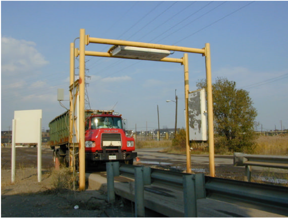
Fig. 3. A portal truck monitoring system commonly used by steel mills to intercept incoming scrap metal. The view shows a truck approaching the monitor, which is located on the approach to the scale. Radiation detector panels are located on both sides and overhead (NCRP, 2002).
